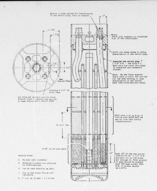
CONCEPTUAL ARPANGEMENT FOR CONVERSION OF "KNOCK-OUT" CANISTER TO A D.E. FILTER WHICH CAN BE USED TO GLEAN UP POOLS & RV
